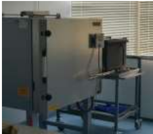
Inert atmosphere heat treatment up to 1200°C
