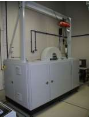
Avure QIH-9 Hot isostatic press up to 3000 Bar (43.5 ksi) and 2000°C
